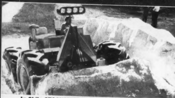
In Chile, STOCKPILES NITRATE —At Port of Iquique, Tournadozer speeds bulk storage and simplifies handling of huge quantities of nitrate while working inside and around the outside of two $8,000-ton capacity storage plants. Big-capacity blade easily moves more than 2½ yards of bulk nitrate on each trip from the conveyor, then rehandles it for delivery through hatchways to dock conveyor. High-speed reverse (8 m.p.h.), approximately twice that of most crawlers, is an important time saver on this shuttle-type operation.
